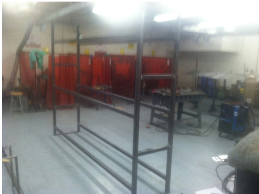
The finished product of the tire rack for Advantage Auto Solution.
