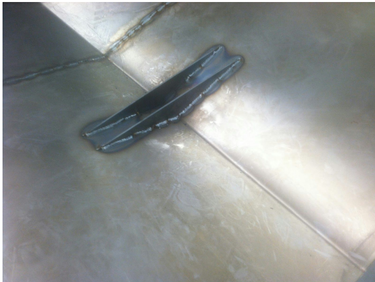
Brackets that Maverick and Alex Taylor have welded onto the Super ATV gas racks roof to stay at a certain angle.
