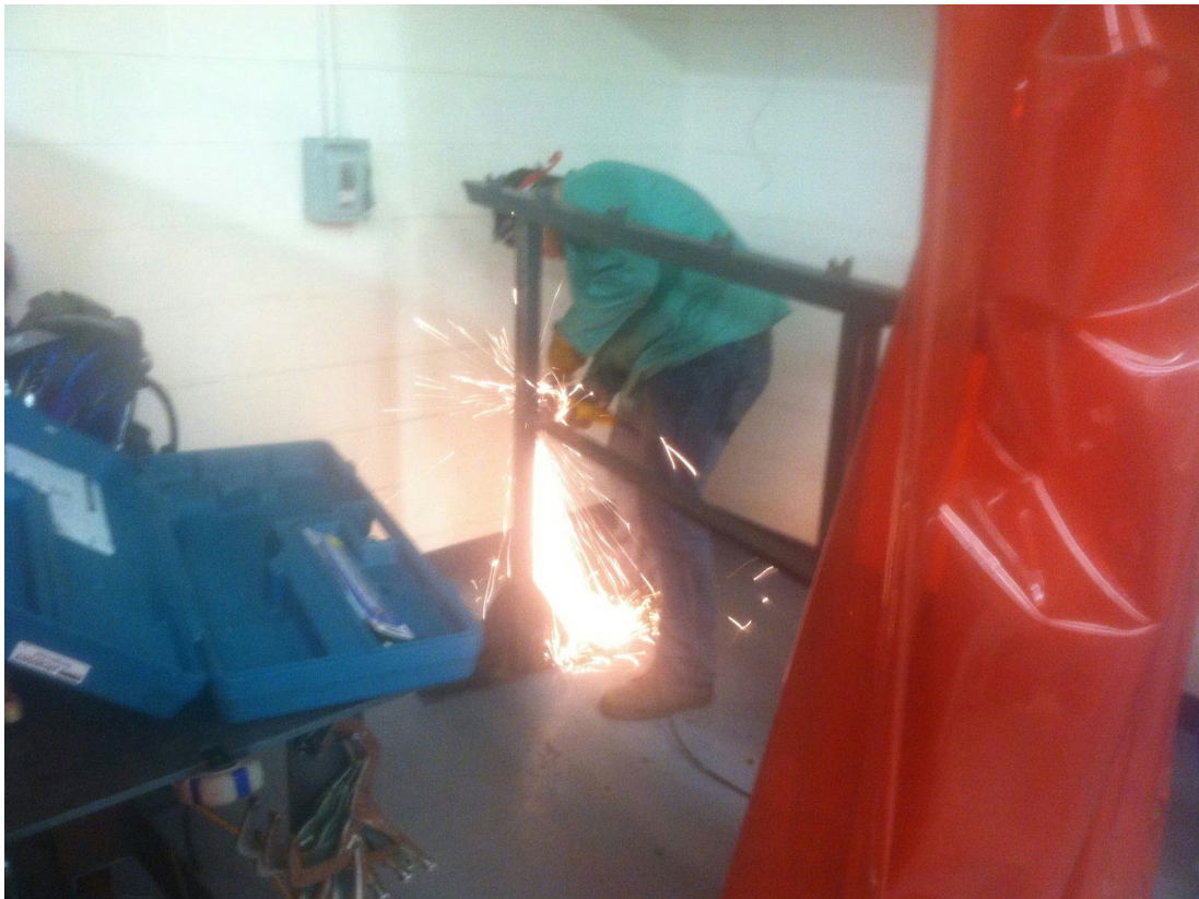
Maverick grinding the last of any excess material off before we start welding on parts for the Super ATV gas rack.
