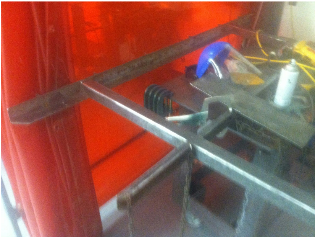
Frame of the SuperATV gas canister rack after grinding was completed.
